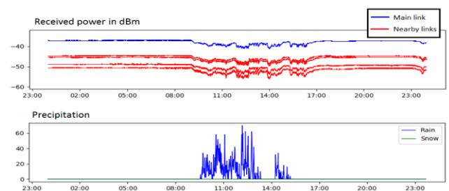
Fig. 1 – Received power over time for a microwave link in Gothenburg, Sweden, showing attenuation during a storm event.
