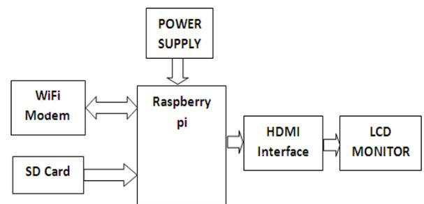
**Fig-1** Block Diagram of IoT based Web Controlled Notice Board
