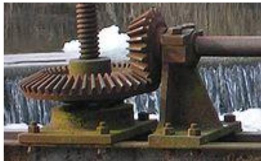
**Figure 4.6.** Bevel Gear
