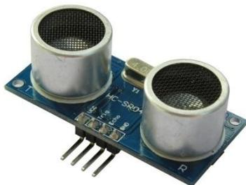
Fig 3: Ultrasonic Sensor
