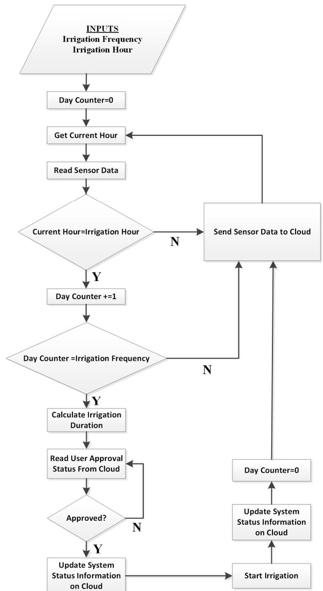
Fig. 1. Block Diagram of the Irrigation System
