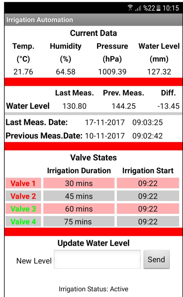
Fig. 2. Screenshot of the Android application taken during irrigation. Valve 1 and Valve 2 are closed. Valve3 and Valve 4 are open.
