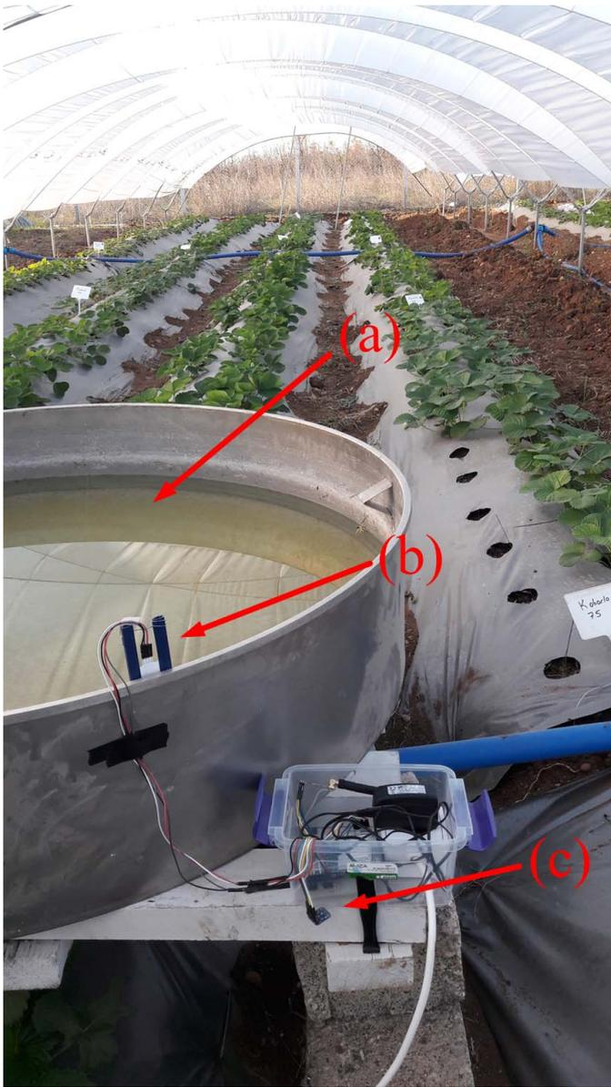
Fig. 3. Data gathering unit inside the greenhouse. (a) Evaporation pan, (b) Water level sensor, and (c) Environmental sensor.
