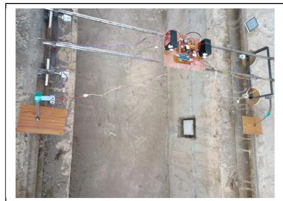
Figure 2. Technical railway crack detection system
