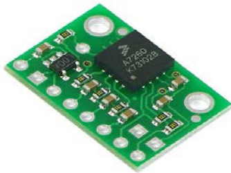
Fig. 7. Accelerometer sensor MMA7260QT
