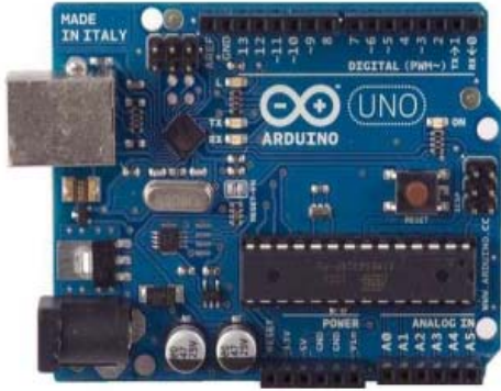
Fig.1 Arduino Uno board with Atmega microcontroller.
