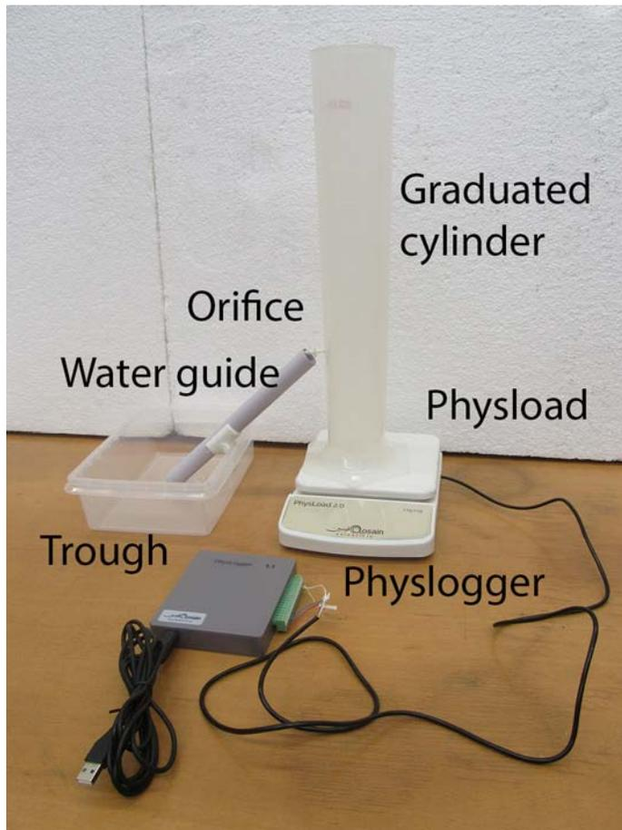
Figure 5: The experimental assembly for observing the rate of discharge from a graduated cylinder.
