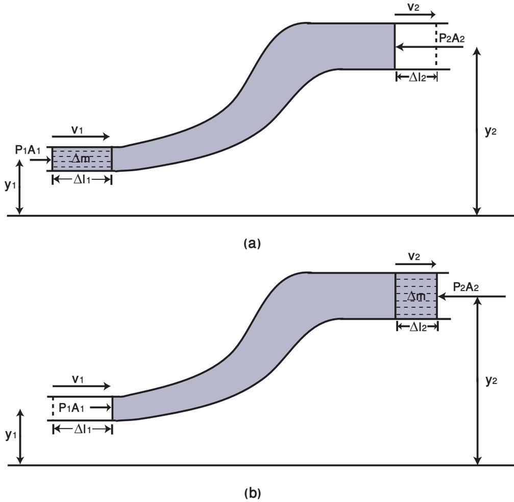
Figure 2: A fluid is flowing through a pipe from position (a) to (b). The net effect is the transfer of the element ( $\Delta m$ ) from the left to the right end. We calculate the work done in this transfer process.
