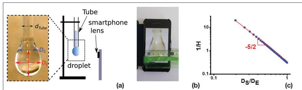
Fig. 1. (a) Water droplet suspended at the tip of a Pasteur pipette. (b) Illustration of the measurement of the diameters directly on the screen of the smartphone with a simple ruler. (c)  $1/H$  as a function of the ratio  $D_S/D_E$ .<sup>10</sup> Note the logarithmic scale on the axes.
