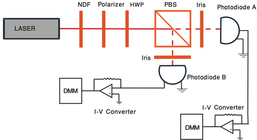
Figure 1: Setup for the experiment. The red line shows the perceived light path.
