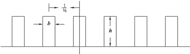
Fig. 1.3. A rectangular wave of period  $1/\nu_0$  and pulse-width  $b$ .
