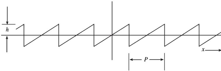
Fig. 1.9. A sawtooth waveform, antisymmetrical about the origin.
