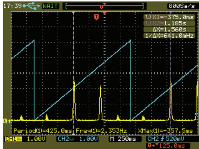
Figure 2: Longitudinal modes of the HeNe laser as seen on the digital oscilloscope.
