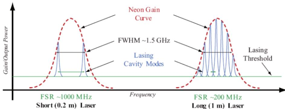
Figure 3: HeNe laser gain curves with longitudinal modes for short and long cavities (HRR020 Manual figure 2).
