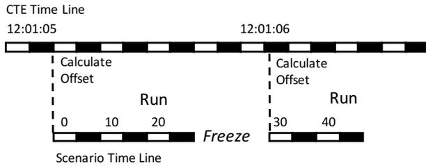
Figure 9: CTE time line and Scenario time line
