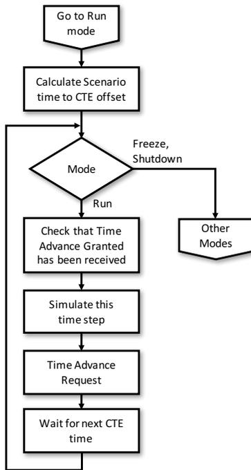
Figure 10: Advancing scenario time vs CTE time
