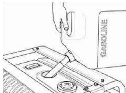
6. Screw on the fuel cap and wipe away any spilled fuel.
