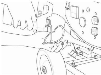
3. Add oil and replace oil fill cap/dipstick. See "Specifications" for oil recommendations based on operating conditions.
