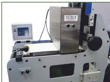
Inkjet Solutions i-JET600 Label Mono print head
