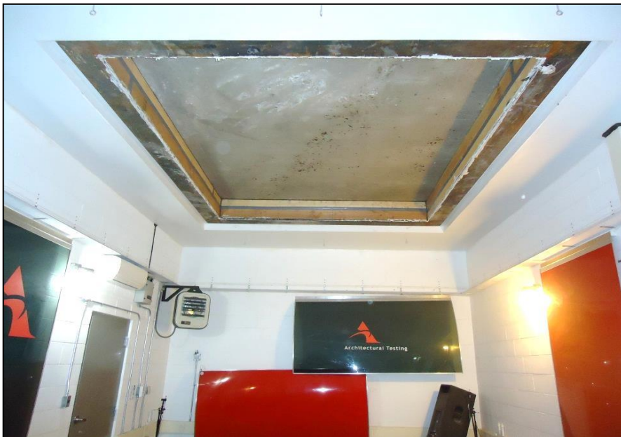
Receive Room View of Test Specimen Installation
