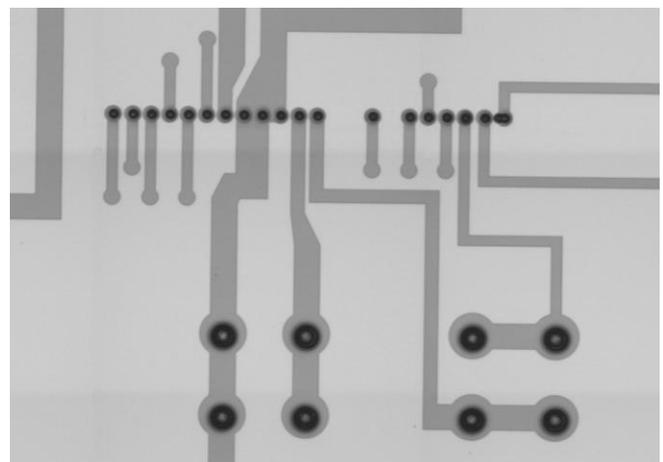
**Figure 1. Automated Inspection Scan of interconnect layer routing over the IC components on the HSIP embedded interposer fabricated for the DARPA ACT program. The image shows good alignment of the first HSIP layers to the embedded IC component.**
