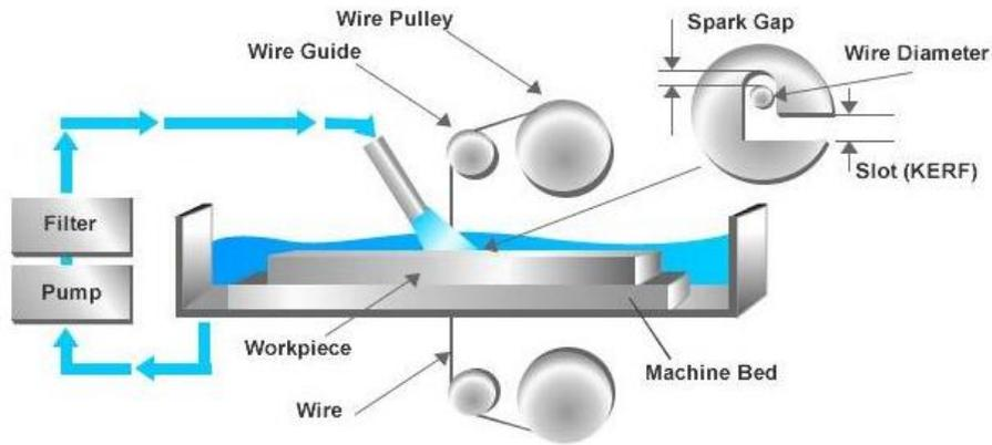
Figure 1. Wire EDM process [7]
