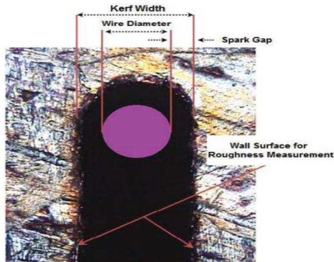
Figure 2. Measurement of surface roughness [18]
