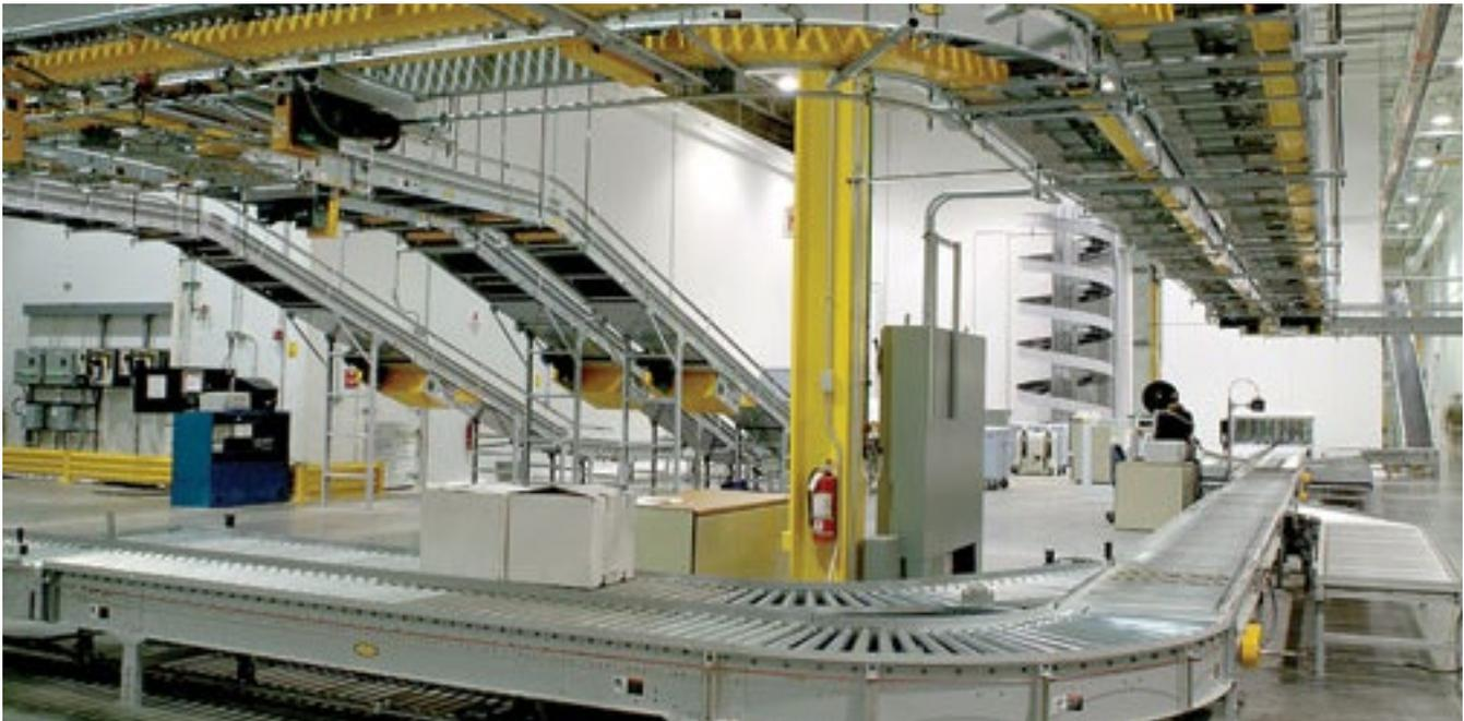
To protect from catastrophic loss of the DC's entire inventory, WEPCO built in redundant equipment at all phases of the operation. That included double conveyor lines, double freezers, double picking zones, double material handling equipment, and two separate electric power feeds from two different substations. Although this drove up construction costs, the value of the inventory justified the investment.
