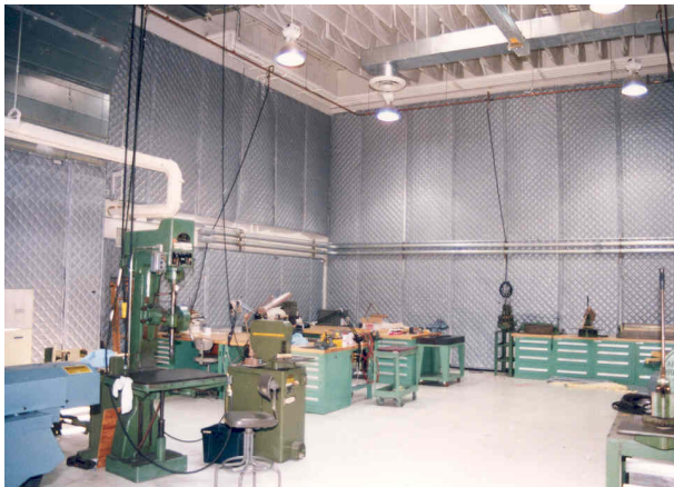
Model QAB-200-VM panels in a fabrication shop effectively control reflected noise.
