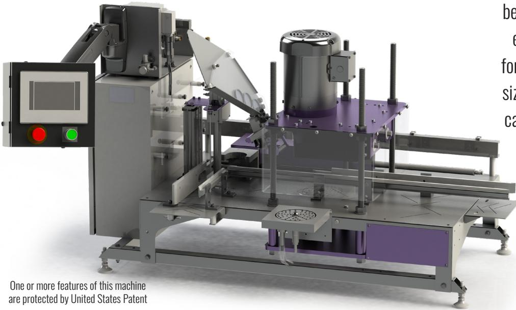
**The Mancos** is designed to give craft beverage makers the nano-canning experience they've been waiting for. No other canning system of any size can deliver on as many varying can diameters, such as sleek, slim, standard and the Crowler™ on one single machine.
