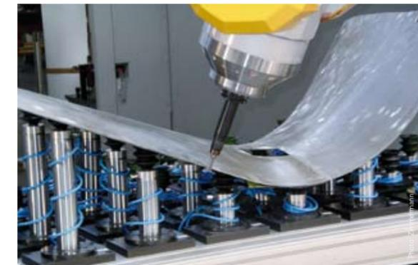
*Part of an Universal Holding Fixture configured specially for securing large, thin-walled or unstable workpieces. Whenever a workpiece change takes place, the fixture is flexibly adapted to the geometry of the new component.*
