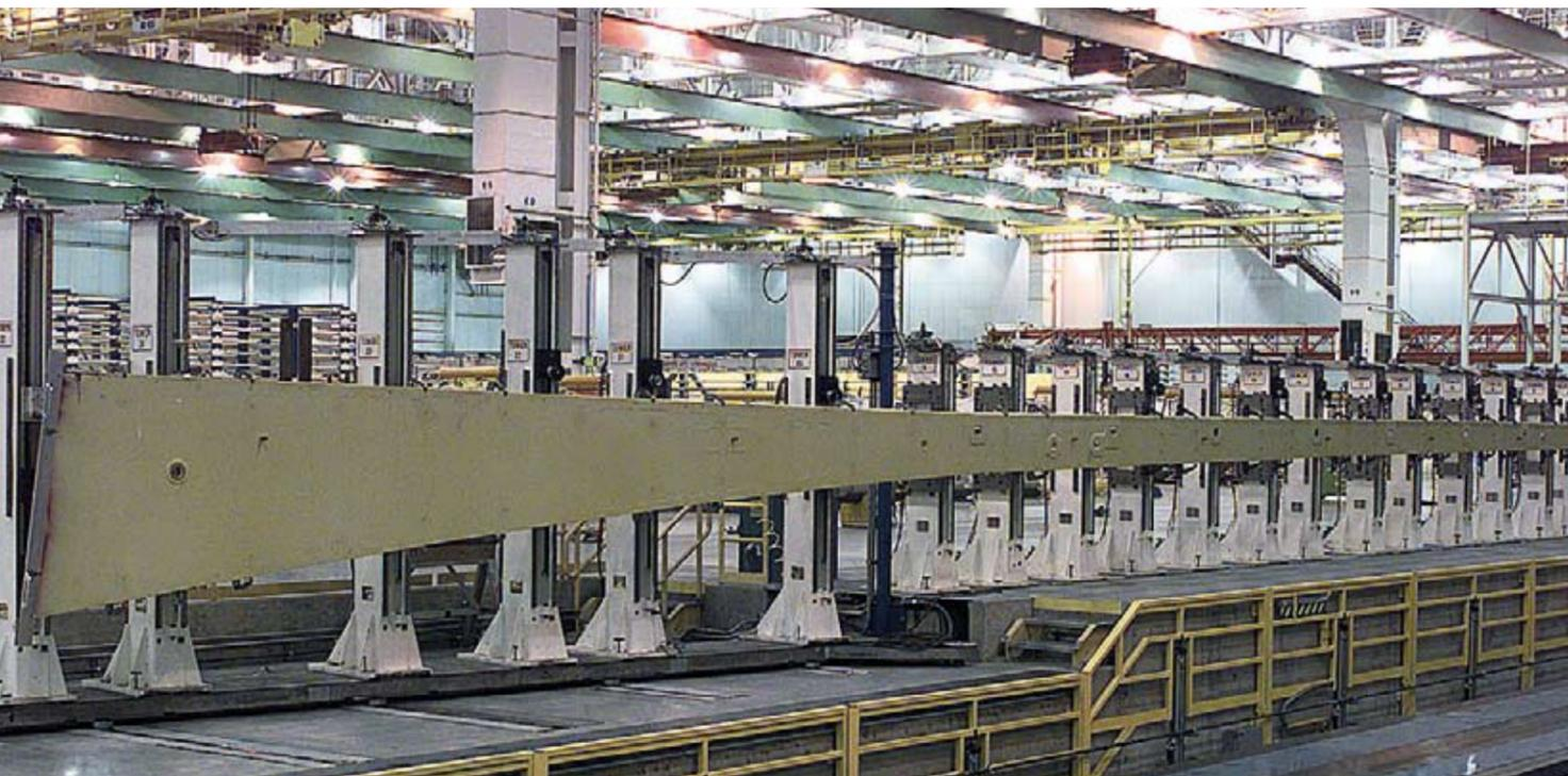
*Clamped wing spar on KOSTYRKA passive UHF.*
