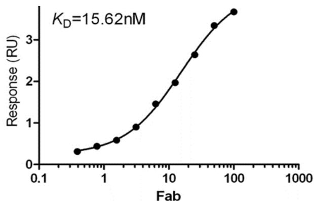
Titration curve of CD64 on a Fab-modified SPR chip.
