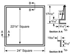
4. For ceilings supported by inverted channel main runners on 24" \mathbb{T}, trim or shear the Therma-Fuser diffuser and use Acutherm hard ceiling frame. Some concealed spline ceilings are hung from inverted channel main runners. If these runners are on 24" \mathbb{T}, remove 4 tiles, remove adjacent cross T's and attach the hard ceiling frame to the main runners with screws. The Therma-Fuser diffuser lays in the hard ceiling frame and provides access above the ceiling without removing tiles.
