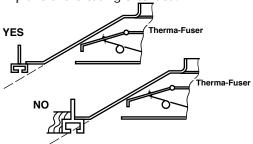
Note: Therma-Fuser diffusers can often be laid on box type without breaking the plane of the casing extended.
