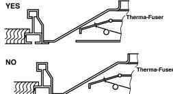
3. Screw standard Therma-Fuser diffuser to bottom of T-bars.
