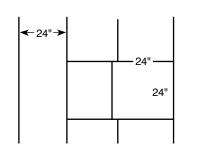
2. Either bevel or cut back ceiling material by <sup>3</sup>/16" on each side to obtain a 22<sup>3</sup>/8" x 22<sup>3</sup>/8" opening and screw the Therma-Fuser diffuser to the joists. Drill two holes in each Therma-Fuser diffuser lip on two opposite sides taking care not to scratch the paint. Use white precoated screws.
