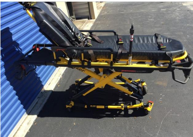
A Power-PRO XT powered ambulance cot made by Stryker is shown
