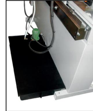
External coolant tank with pump
