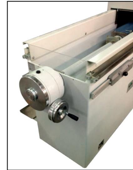
Angular divisor for magnetic chuck  $\pm 90^\circ$
