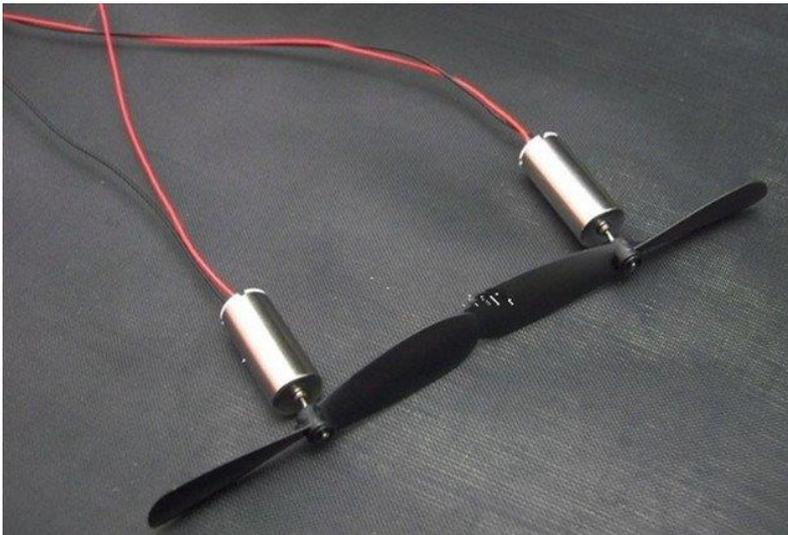
These are the type of motors having high rpm (rotations per minute) i.e., approximately 22,000 rpm. They consume about 3.5V-4V and 2A of current for its efficient performance. In our project we are using 4 motors, 2 for propulsion and 2 for pressure.
