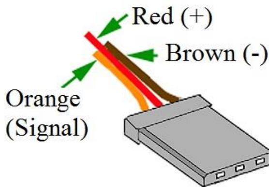
Servos are devices that are commonly used in robotics and have many applications. Servos are used to move object parts from one angle to another and most servos can only move within a limited range. In order to assess how far a servo can move, the gears inside the servo must be examined. In addition, the servo may have a tab to help the servo define the limits of rotation.
