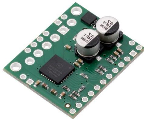
This is a type of circuit which increases the amount of voltage. In our project we used it because it takes 3V as input and gives 5V as output. This is used to drive 5V to give it as power supply to Arduino Nano and stepper.
