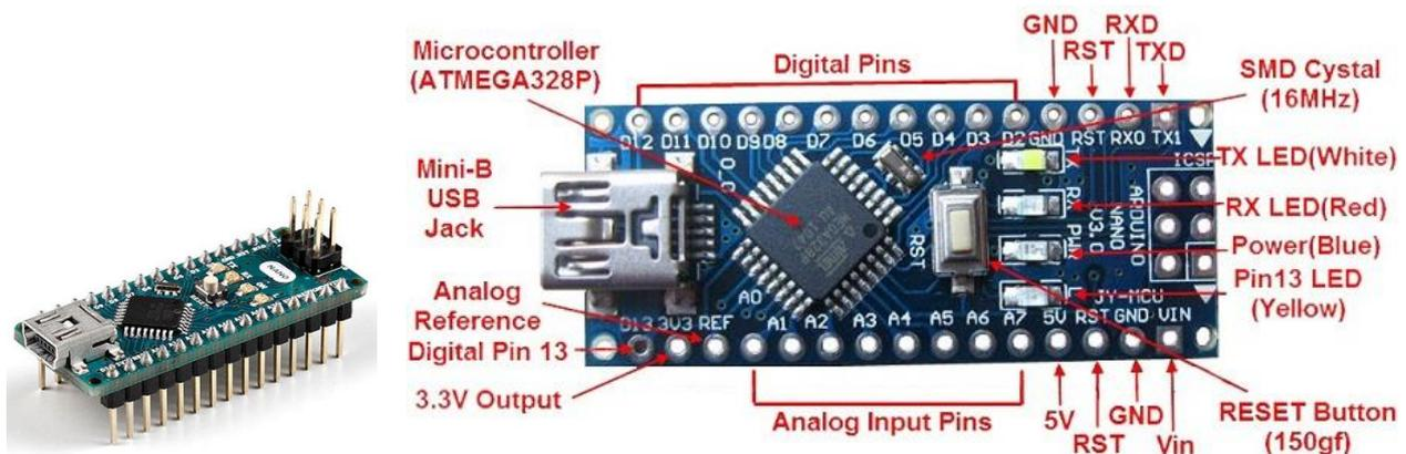
The Arduino Nano is a small, complete, and breadboard-friendly board based on the ATmega328; offers the same connectivity and specs of the UNO board in a smaller form factor.
