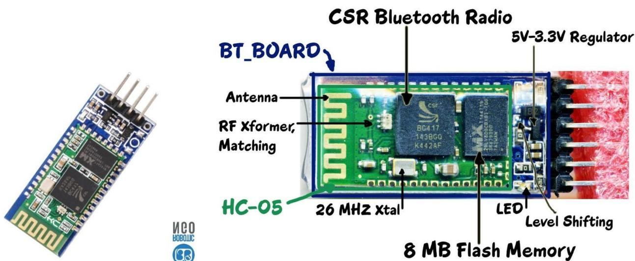
**HC-05** is a class-2 **bluetooth module** with Serial Port Profile, which can configure as either Master or slave. a Drop-in replacement for wired serial connections, transparent usage. You can use it simply for a serial port replacement to establish connection between MCU, PC to your embedded project and etc.
